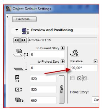
Horizontal structures are created with ArchiCAD slab tool. Panel direction is set to object tool's default settings in *Object angle*. To edit angle, please recreate the panels for the slab.
