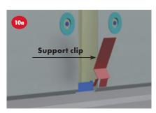
10 Fix a support clip to the external flange of the U-profile. Remove all the silicone paper, also in the middle. Attach the foil carefully to the support clip and the outer flange of the U-profile. (Pictures 10 a-c)
