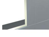
The top end of the cover flashing is fastened with pop rivet if it not locked into a panel joint.
