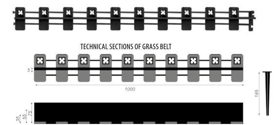
The edge is assembled with the use of connectors, it is stabilised in the ground with assembly pins. Made from high-quality plastic (polypropylene) and are characterised by high quality, durability and resistance to atmospheric conditions.
