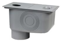
The drain cover is composed of the spout cover and full cover. The spout cover has pressed spots ready to prepare openings for spouts/pipes diameter Ø 50, Ø 80, Ø 90, Ø 100, Ø 110mm. Full cover enables inspecting and removal of dirt. The body of the under spout drain has a vertical outlet for sewage pipes diameter 110mm. Inside there is a basket preventing the dirt from entering the sewage system and an anti-odour lid.
