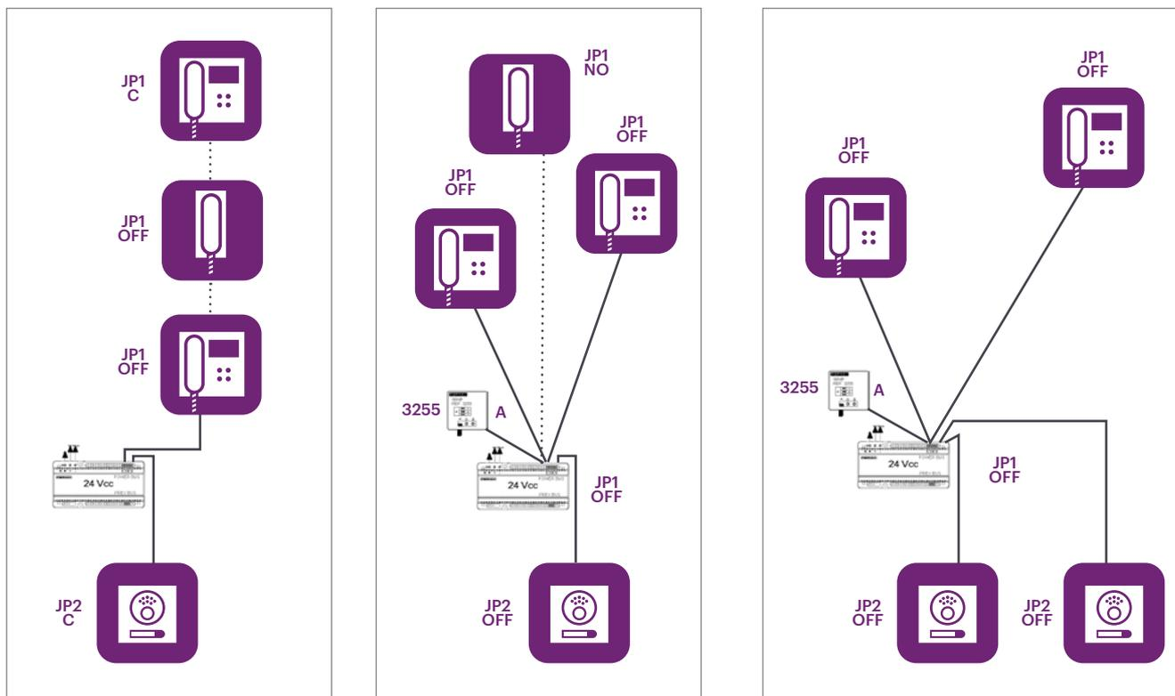
**INDOOR:** The kit allows a maximum of 3 terminals (the included one and 2 additional ones). Depending on the type of cable and distances, an additional power supply (ref. 4825), line adaptor ref. 3255 and/or regenerators might be required.
