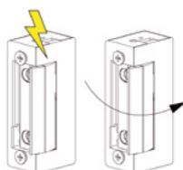
Allows door opening while power to the lock release is off.
